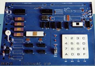
The CDP1802 8-bit microprocessor combines CMOS technology and the elegant COSMAC architecture. These features have made it the choice in a wide range of applications. TV games. Automotive engine control. Factory automation. The CDP1861 chip provides a video-frequency output signal with sync and was especially designed to interface the COSMAC CPU to a low-cost TV monitor.
